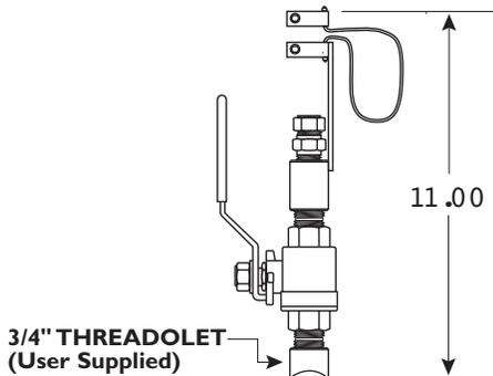
**NOTE:** User needs to weld a 3/4" female threadolet (of appropriate radius) to mate with existing pipe after a 3/4" hole has been drilled in pipe. The 3/4" Male Coupling of the Sage Isolation Valve Assembly will thread into the user's 3/4" threadolet.
