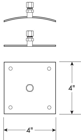
1 At 650 psig, force exerted on 1/2" diameter probe is approx. 125 lbs
