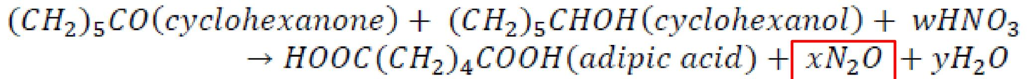
Adipic acid  $\text{N}_2\text{O}$  abatement or control technology can be installed downstream of where the reaction occurs to treat the facility's off gas
